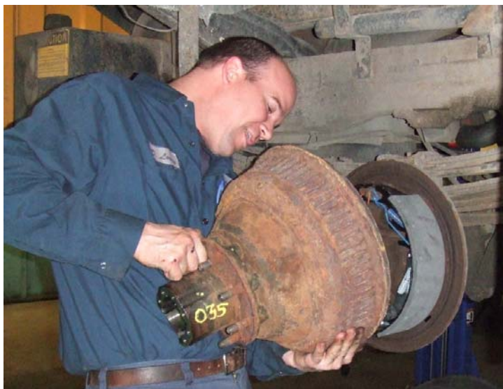
David Lowry completing the installation of the rear brake drums after performing a 4 wheel brake job.
