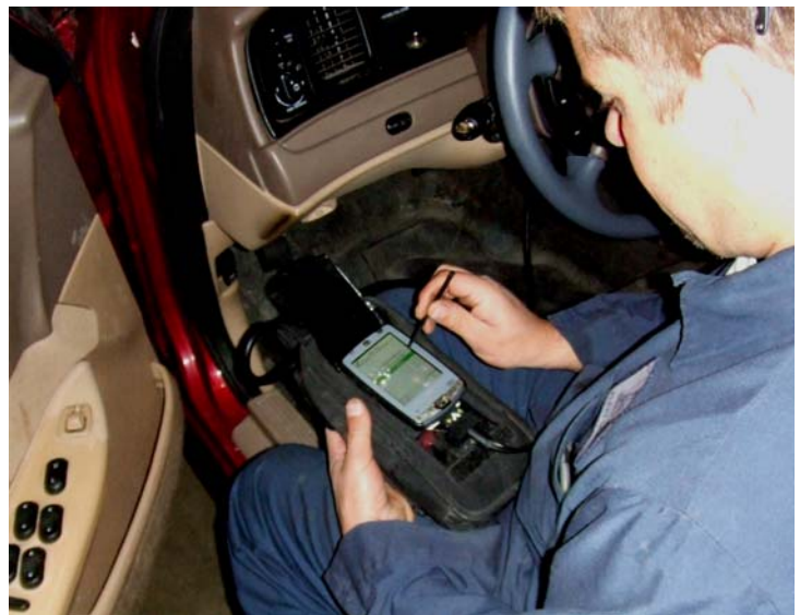
Brad Morin using the PDF scanner to check the vehicles computer diagnostic system
