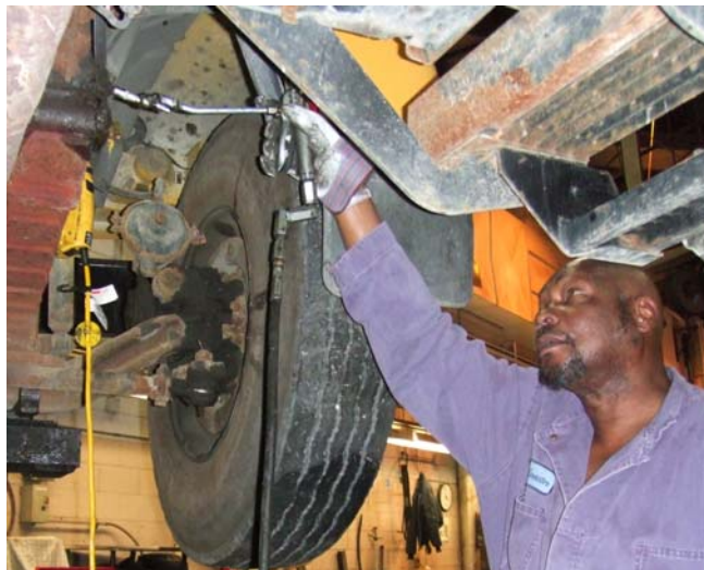
Ron Caracter lubricating a suspension during preventive maintenance
